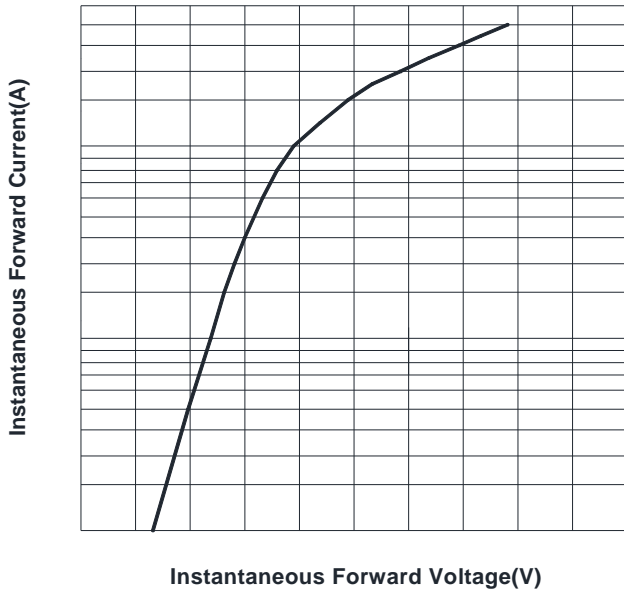
FIG3: Typical Forward Voltage
